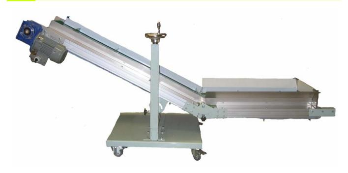
The CC Pedestal Conveyor is a conveyor designed specially for the Plastics Industry. It is free standing and mobile and can be made into many configurations to suit injection moulding machines.
